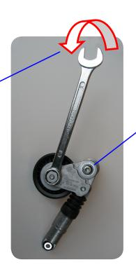
The tightening torque on the bolt bracket is 25 Nm.
